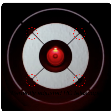
well aligned RC telescope
