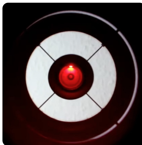
RC telescope with correctly adjusted secondary but misaligned primary mirror.
