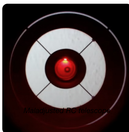
misaligned RC telescope
