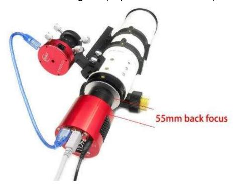
Mono camera connection diagram (depicted with EFW, OAG& Guide camera):
