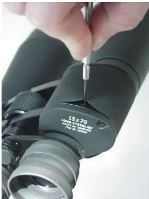
The setscrews move the image in the same direction as the screw. So when screwing the right setscrew inward (clockwise as viewed from above), the right image will move downward and also to the left. Unscrewing the right setscrew (counter-clockwise) moves the image upward and also to the right.
