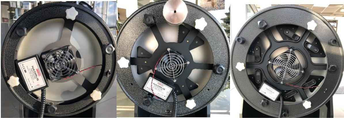
Examples of electronic box mounting on GSO 10", 12", 16". 8" Dobsonian can be used, but the fan has to be removed from the primary mirror cell to leave enough space to the electronic box.
