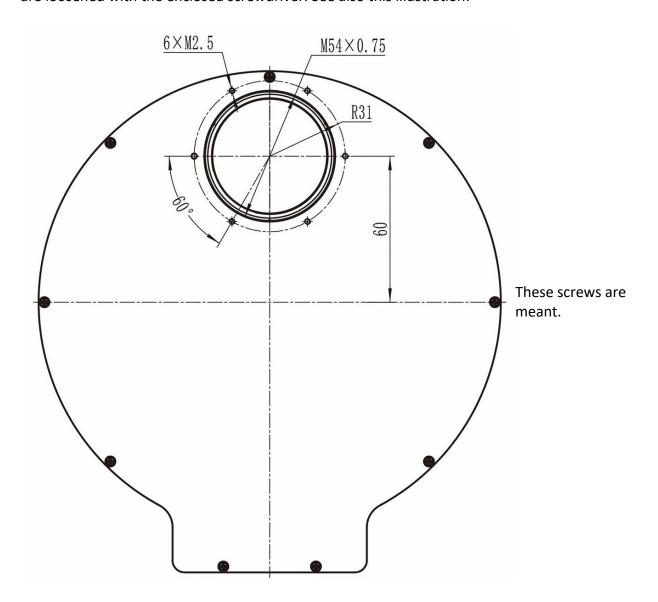
The cover plate can now be removed and the filters are accessible. The camera can stay mounted.
