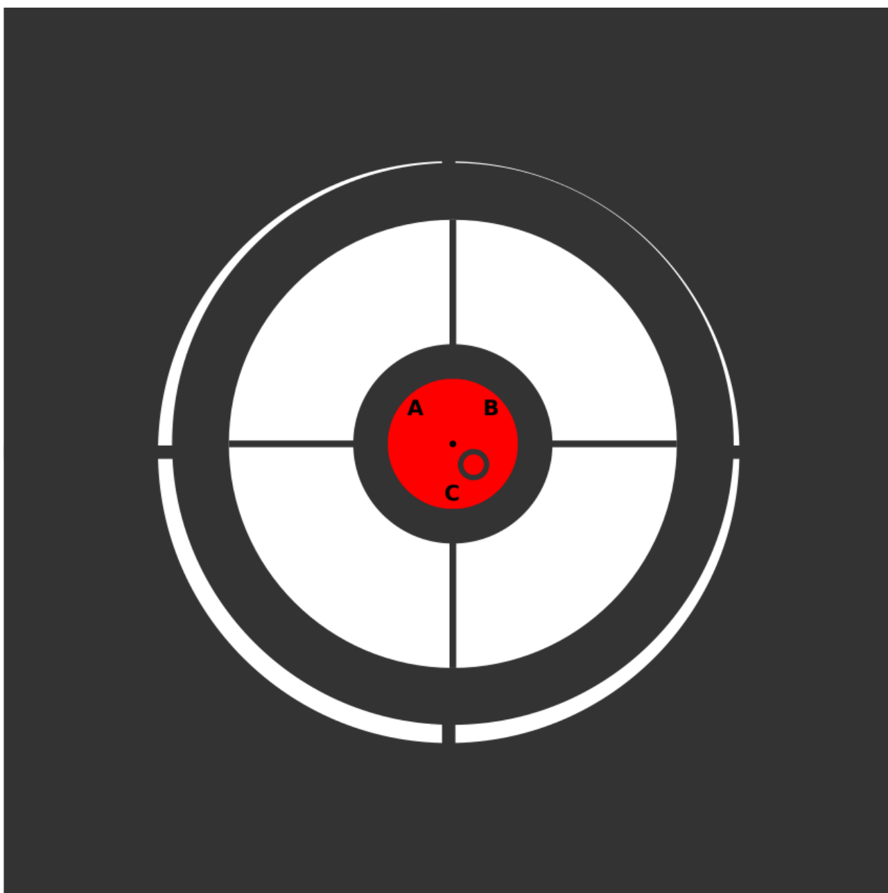
Depiction of a mis-collimated RC telescope.
