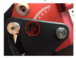
Turn the Latitude Adjustment knob all the way up. Then turn the lower eyebolt all the way up. Adjust the lower eyebolt so that the hole is facing sideway.
