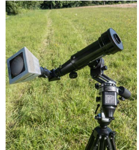
Celestron TravelScope, with 18mm Classic Ortho, stopped down, on a lightweight travel mount. OPFA at 1¼" mirror diagonal
