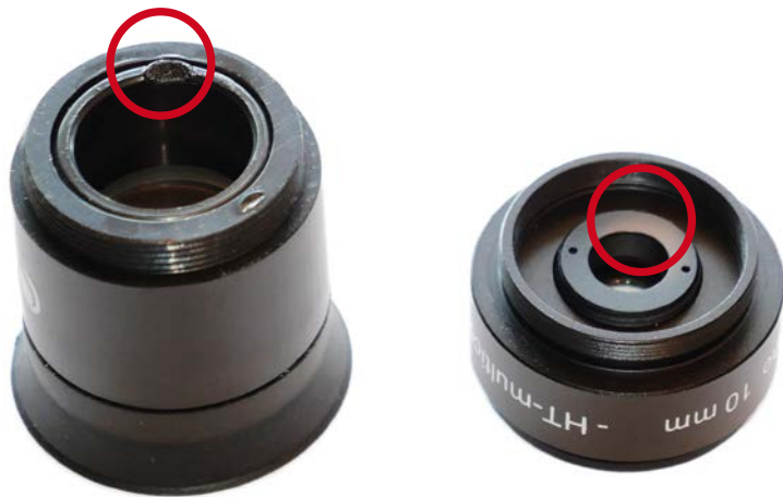
Left: A cheap eyepiece with plastic housing shows scorch marks even after the Sun was out of the center just for a short time.
