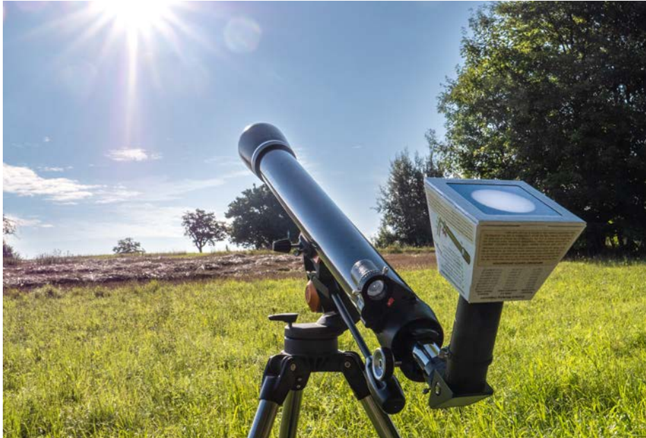
Celestron AstroMaster 70/900AZ, with 18mm Classic Ortho. Due to the back focus, the OPFA is mounted directly at the prism diagonal #2456005
