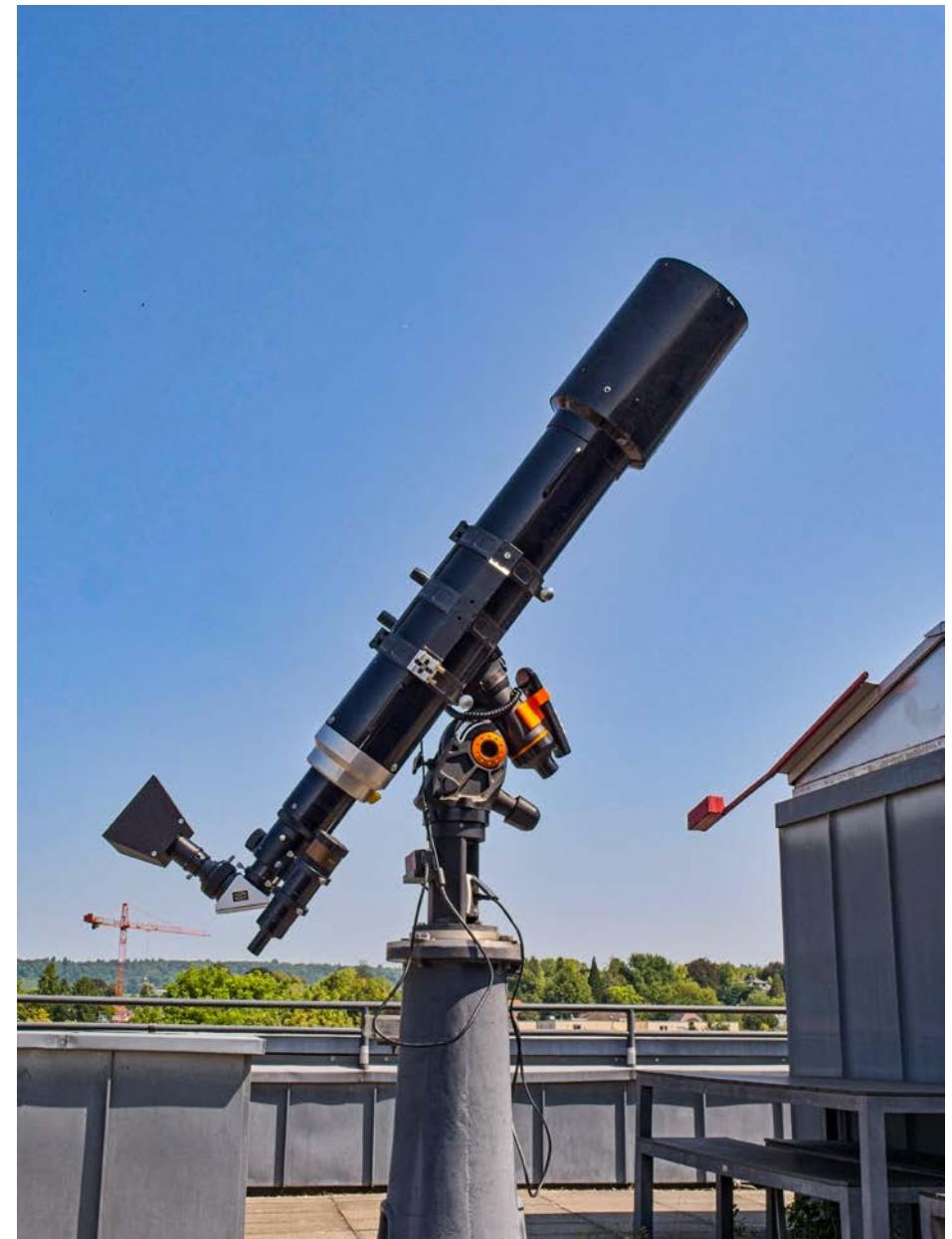
The Solar Projection Screen on a 150/1200-telescope with the 3D-printed housing.
