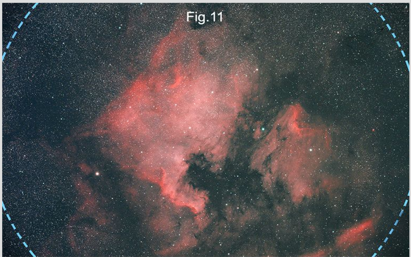
Fig.11 This image representing NGC 7000 clearly shows the vast field encompassed by the SQA as well as the very discreet vignetting on the edges.,Ten minute expose with IDAS NBZ filter where only the contrast has been increased to show this vignetting. You can notice that the image is fully usable
