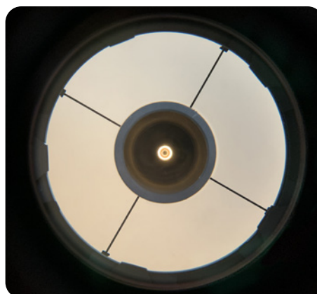
Adjusted RC telescope, TSCOLLIT-G2 focused on secondary mirror spider.
