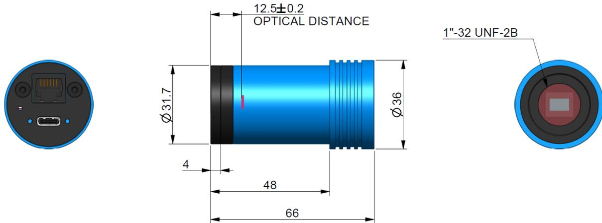
Figure 5 Dimension and Mount of GPM462M and 1.25" extender
