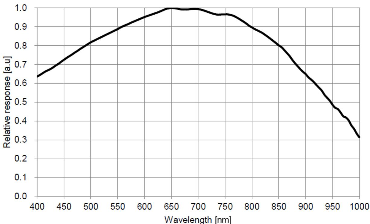
Figure 1 IMX462 Spectral Sensitivity Characteristic
