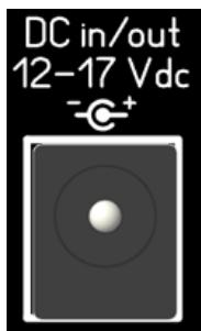
There are two DC input/output ports: one located on the front side of the controller and another on the back side.
