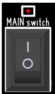
The main switch allows you to turn the controller on and off. The LED above the main switch indicates the current status of the controller.
