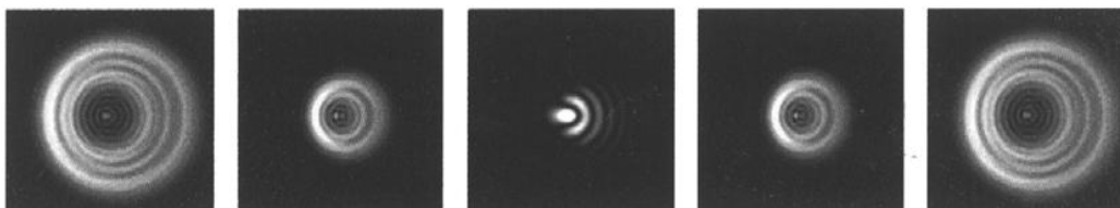
Figure 8-2 -- Even though the star pattern appears the same on both sides of focus, they are asymmetric. The dark obstruction is skewed off to the left side of the diffraction pattern indicating poor collimation.
