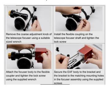
Note: You can use any thread which the focuser have to attach the L-bracket of the EAF. Don't forget to remove the focuselockscrew, you don't need it anymore when the autofocuser is attachet.
