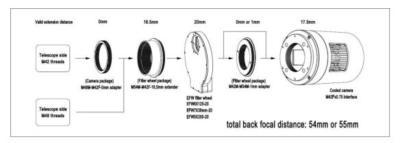
Figure 7 Connection with ToupTek cooling camera
