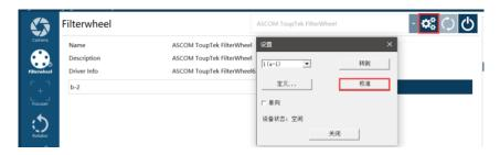
Figure 14 ASCOM filter wheel calibration
