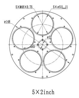
Figure 6 Filter disk 5x2" front.
