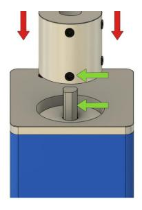
To create an optimum connection between the AAF motor and the flexible coupling, align the adjacent screw with the flattened shaft. (see green arrows)
