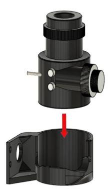
Place the AAF adapter on the table and slide or press the focuser into the adapter from above as shown.
