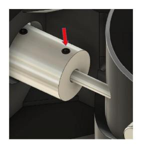
In the last step, screw the two grub screws oft he coupling to the focuser.
