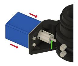
Then connect the motor to the coupling using the AAF adaptation. The coupling must be pushed onto the shaft.
