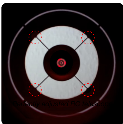
Well-adjusted RC telescope
