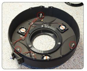
Now place the back plate on the edge of your work surface so that the position of an collimation screw is accessible from below. Hold the screw-spring pair in this position and remove the associated adhesive tape. Use the appropriate Allen key to hold the screw in place.
