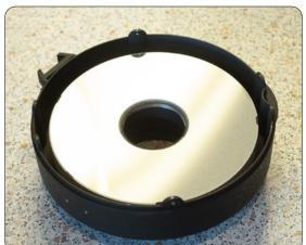
Connect the retaining ring and the baffle tube and screw the assembly onto the carrier. As soon as you feel a greater resistance, check whether the mirror can still be moved. It must still be easy to turn, but under no circumstances should it be possible to tilt it.
