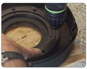
Remove the ring and widen the 3 mm hole to 8 mm.
