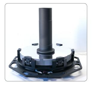
Place the back plate with the cell on a protective surface and remove the baffle tube. Take care not to touch the mirror.
