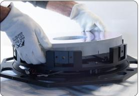
Carefully place the mirror upside down on the felt glides and remove all adhesive residue with the scraper, a suitable solvent (spirit, isopropyl alcohol or similar) and cloths. Even if it is the back, do not use any metal tools!
