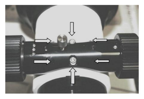
Next, tighten the four recessed grub screws to the left and right of it (horizontal arrows) a little.
