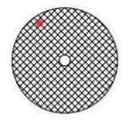
Step 6: Loosen adjusting knob ① on the back cover plate, and turn adjusting knob ② to change the tilt of the primary mirror. Adjust until the laser dot is perfectly centered on the reticle of the collimator:
