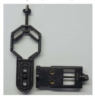
The adapter consists oft wo parts: the eyepiece part (left in the picture) and the smartphone holder (right in the picture). The smartphone holder can be mounted in two heights using the brass thread bores, according to the length of the phone. Additionally, it can be mounted with the locking screw to the left or to the right, depending on the position of the lens on the phone.
