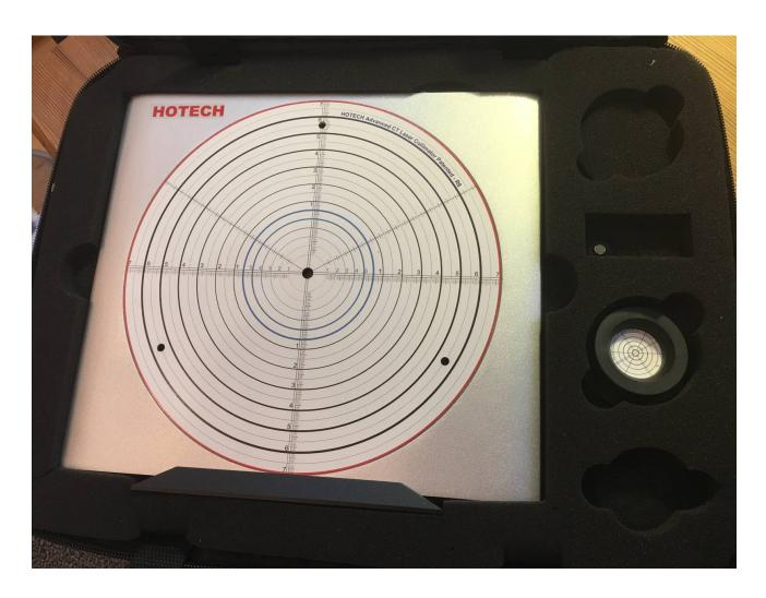
This is for the standard SCT version. You also get an adapter that places a semi-transparent mirror in the focal plane of the HyperStars and a cap with a centering disc. The cap with the centering disc can be used up or down. This is required in the individual collimation steps.
