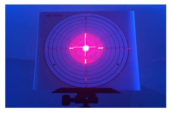
The two crosses must be aligned using the tension and compression screws on the HyperStar.
