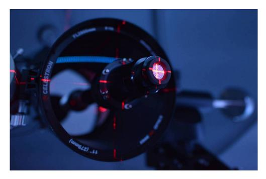
If the point is in the middle of the centering disc, then the collimation is done. Otherwise the corrector plate must be adjusted.
