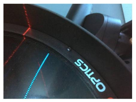
Use a small Phillips screwdriver to loosen the screws so that the ring is on the corrector plate no longer exerts any pressure. Then you can adjust the corrector plate alignment using the four Allen screws located on the side of the tube.
