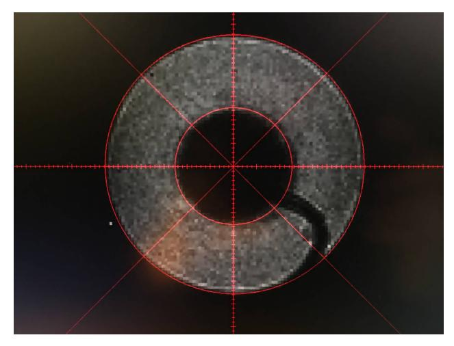
You can also check the collimation, using software such as CCDInspector or the WaveformEstimator in PixInsight.
