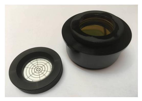
Now you can see another cross on the target of the collimator. If the new cross is shifted in relation to the cross of mode 1, then a collimation is necessary.
