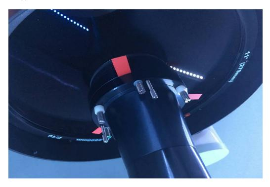
The actual collimation of the HyperStar is very simple. Remove the camera and place the Hyperstar adapter. Start by unscrewing the centering disc from the HyperStar adapter and set the collimator in modes 2 or 3 (three lasers + crosshairs).
