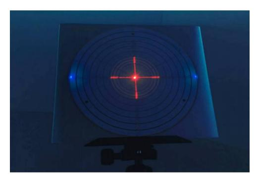
As you can see, a tedious task can now be done just in a few minutes. At this point you should tighten all screws firmly without deforming anything. The collimation is now complete and, in my experience, it lasts for a long period of time. Now you can also switch the HyperStar and the secondary mirrors without loosing the collimation.
