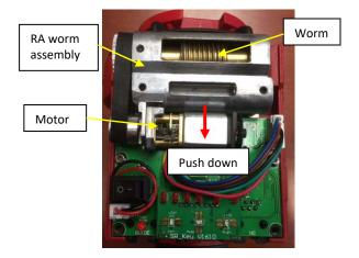
Now without pushing down the motor, rotate the RA axis to check the play. Please pay attention to the worm assembly movement. If the whole box is moving side to side, the hinge is not secured or positioned well.
