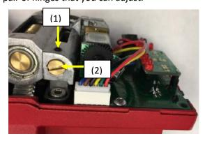
7. If the play is due to RA worm movement, as shown below. You need to tighten the RA worm, which needs to remove the worm assembly.
