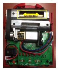
8. If neither the worm nor the assembly is moving, the play may caused by the worm is not centered on top of the ring gear. The worm box needs be adjusted.
